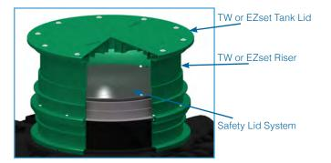
3. Disassemble the riser stack and Safety Lid System. Apply generous amounts of sealant on each surface and reassemble the riser stack and Safety Lid System back into the proper position.
