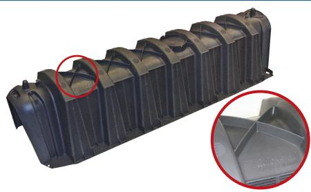
The Quick4 Equalizer 24 HD Chamber was designed to provide exceptional strength when used in heavy duty trench or bed applications. The chamber's enhanced features, which include an increased wall thickness, structural x-ribs and reinforced connection joints, make it one of the strongest Quick4 chambers available today. The Quick4 Equalizer 24 HD Chamber's Contour Swivel Connection permits 15° turns, left or right.
